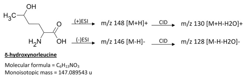
Fig. 6. Identification of \delta -hydroxynorleucine using mass spectrometry. With (+)ESI-MS (electrospray ionization mass spectrometry, positive ion mode), \delta -hydroxynorleucine readily forms a mass-to-charge ratio ( m/z ) of 148 [M+H]^+ , which upon collision-induced dissociation (CID) produced the m/z 130 [M+H-H_2O]^+ product ion. With (-)ESI-MS (electrospray ionization mass spectrometry, negative ion mode), \delta -hydroxynorleucine forms an m/z 146 [M-H]^- ion, which upon CID results in an m/z 128 product due to loss of H_2O . Loss of 46 u and 44 u from the [M+H]^+ and [M-H]^- ions, respectively, as shown in the figure are common for amino acids.
