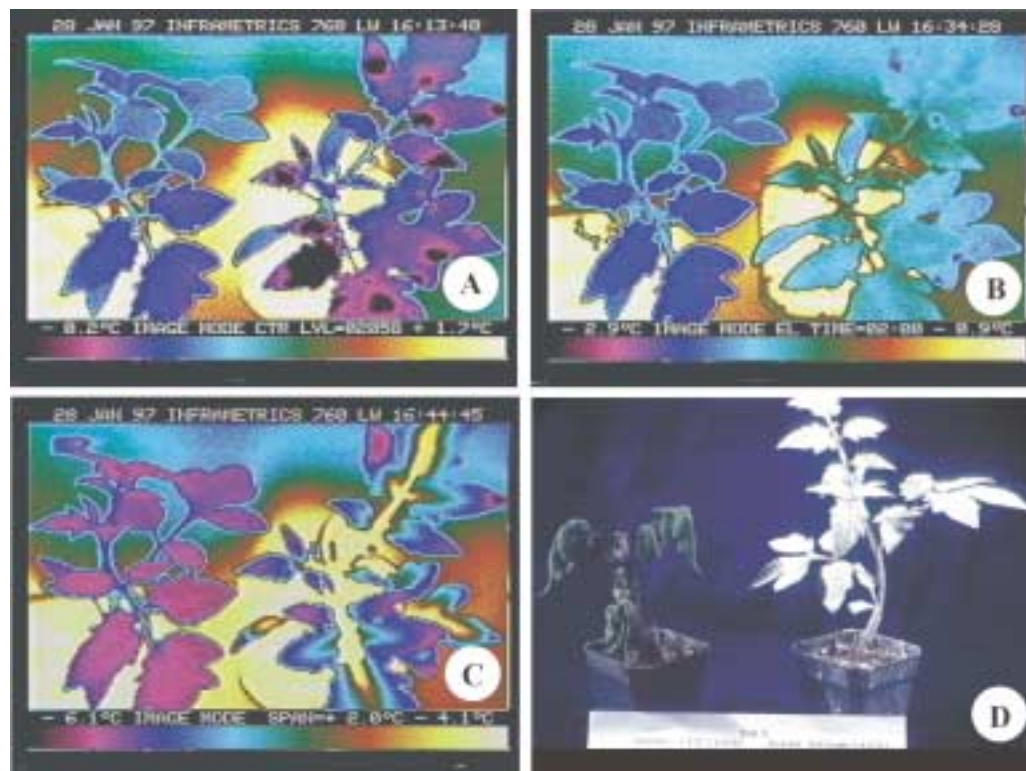
Fig. 6. (A–C) Infrared thermography and (D) a photograph of noncoated and M96-018 coated tomato plants subjected to freezing temperatures. Each plant was sprayed with water containing Ice + bacteria using a hand-operated aerosol sprayer. The coated plant is on the left in (A–C) and on the right in (D). Large drops of water can be seen as black areas on the noncoated plant in A. The black areas are a result of these areas being colder than the set temperature range of the camera (−0.2 to 1.7 °C). The lower temperature of these areas is due to evaporative cooling. In B, the noncoated plant is in the process of freezing, as evidenced by the warmer temperature resulting from the exothermic reaction of ice formation, while the coated plant is unfrozen at about −2.5 °C. In C, the noncoated plant has almost completely frozen, except along the stem, petiole, and midvein, and is approaching temperature equilibrium with air temperature. The coated plant in C is still unfrozen at about −6.0 °C. In D, noncoated (left) and coated (right) plants can be seen after exposure to −6.0 °C, removal from the chamber, and thawing. The noncoated plant is completely killed while the coated plant appears uninjured.
