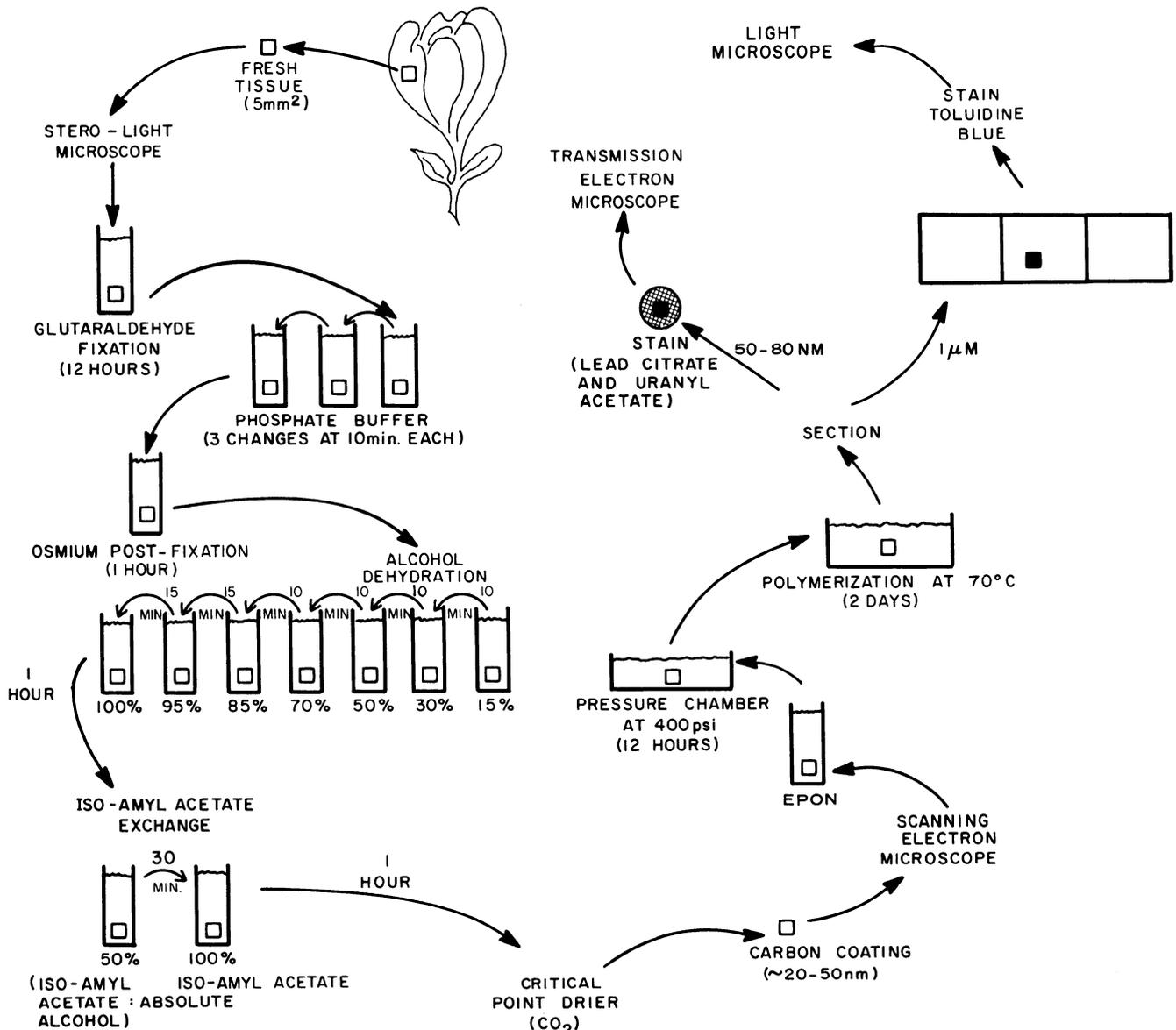
Fig. 1. Schematic diagram of the pressure embedding technique.
