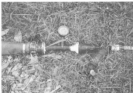
Fig. 14. Simple venturi-type fertigation unit (brass siphon mixer) connected to a hydrant.
