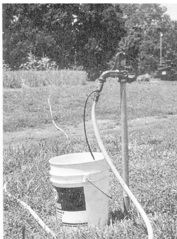
Fig. 14. Simple venturi-type fertigation unit (brass siphon mixer) connected to a hydrant.
