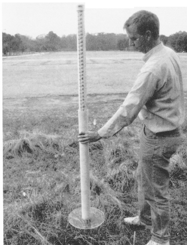
Fig. 1. Disc meter in use measuring unmowed turfgrass.
