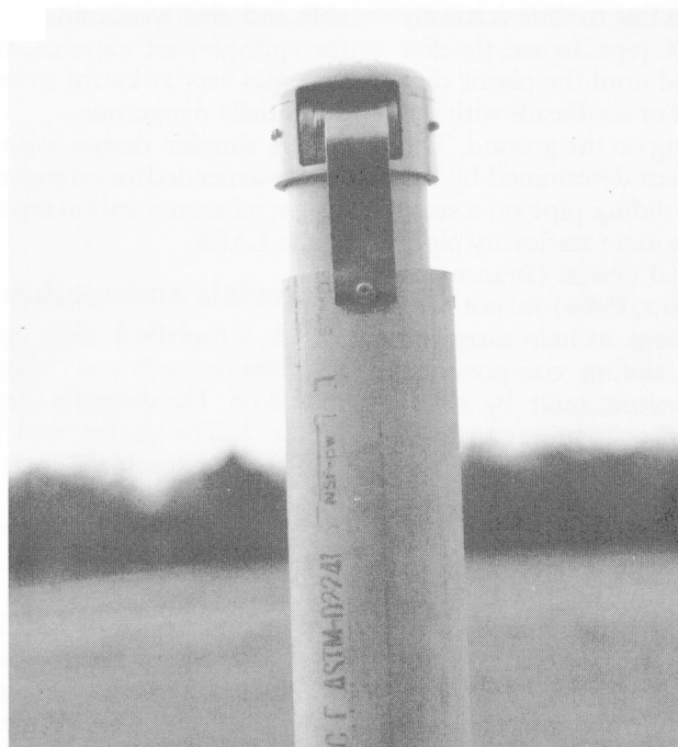
Fig. 2. Detail of constant-force spring mounted on disc meter.
