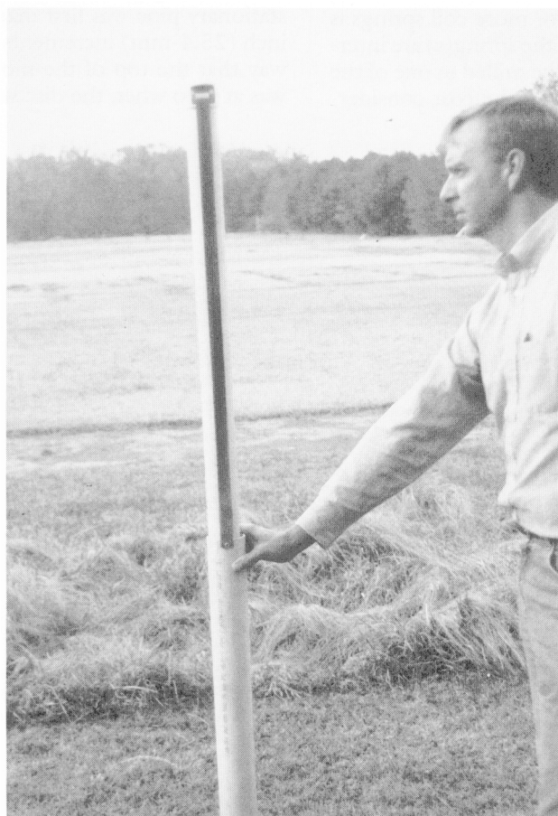
Fig. 3. Constant-force spring extended as measuring disc is lowered.
