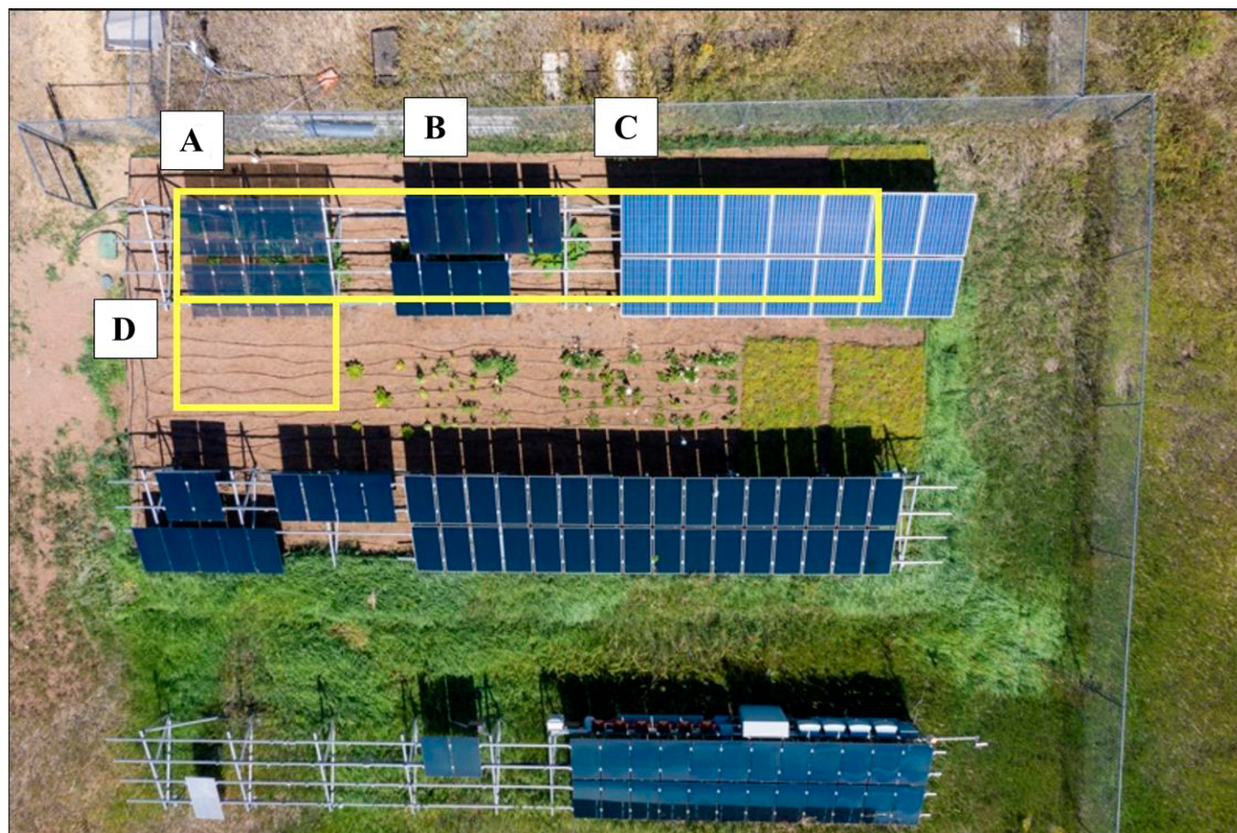
Fig. 1. Solar modules used in this project. Left to right: A, 40% semitransparent cadmium telluride (CdTe) frameless solar modules; B, opaque CdTe frameless; C, opaque polycrystalline silicon module; and D, full sun control. Photo: Matt Staver.
