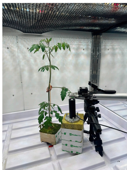
Fig. 2. A setup for leaf photosynthesis measurement using a portable photosynthesis system in a growth chamber and light measurement by a spectroradiometer.
