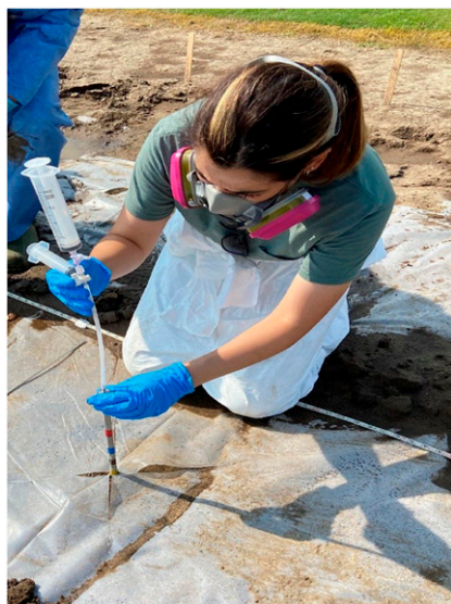
Fig. 2. Soil gas collection using an AMS 12 GVP soil gas probe (AMS™, American Falls, ID, USA) in the tarped treatment.
