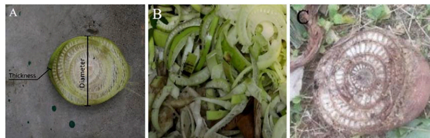
Fig. 5. Effects of the banana pseudostem chopping. (A) Measurement of the chopped pseudostem size, (B) qualified banana pseudostem, (C) unqualified banana pseudostem.
