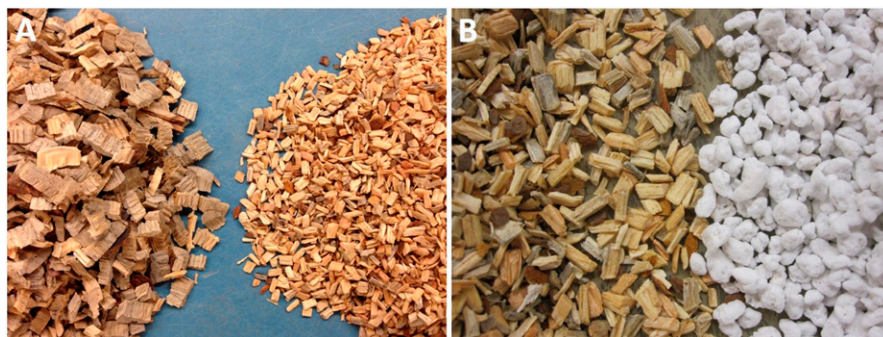
Fig. 1. (A) Harvested loblolly pine logs were chipped in a wood chipper resulting in large wood chips [1.0 × 0.2 × 1.0 cm (length × width × height)] before being milled through a 1/4-inch (6.35 mm) hammer mill screen resulting in (B) smaller pine wood chip aggregates that are square/blockular in nature and contain little dust or fibers and are similar in size to horticultural grade perlite; 1 cm = 0.3937 inch.
