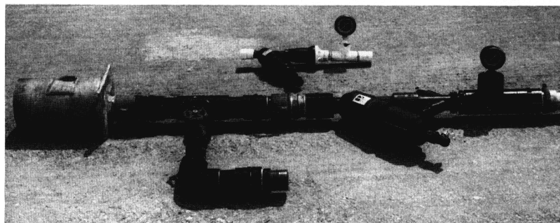
Fig. 1. Two different-size units for use with well water. Each contains a screen filter, pressure reducer, and pressure gauge.
