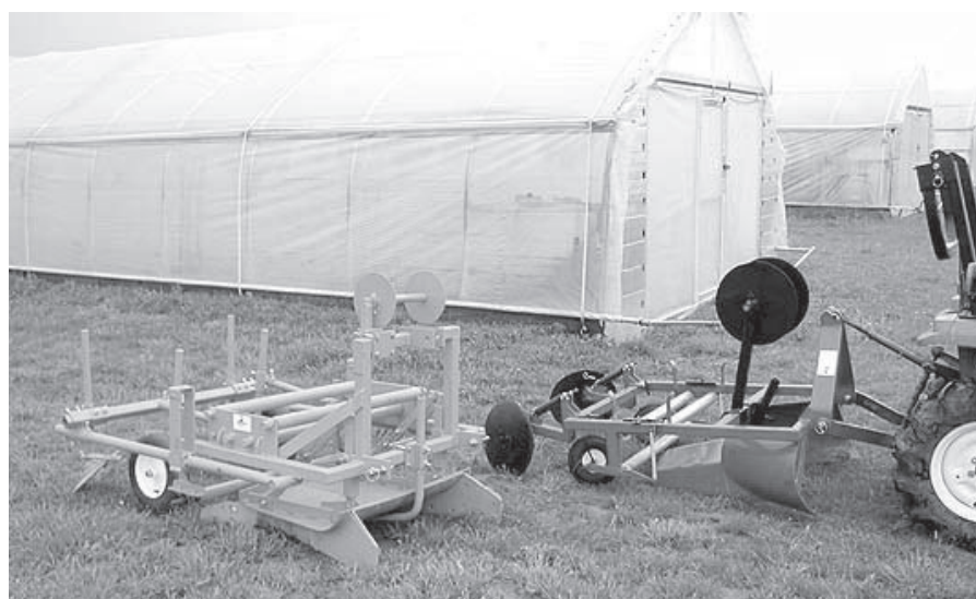
Fig. 3. Small plastic mulch/drip irrigation tape applicators [Nolt's Produce Supplies, Leola, Pa. (right) or Reddick Fumigants, Williamston, N.C. (left)] used to make a 3- to 4-inch (7.6- to 10.2-cm) high, raised plastic mulch covered bed 18 inches (45.7 cm) wide with a drip irrigation tape.
