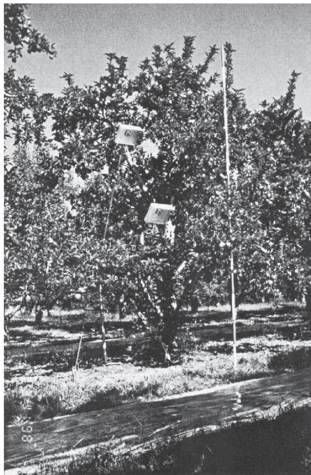
Fig. 2. Quantum light data loggers (model 3600; Spectrum Technologies, Inc., Plainfield, Ill.) positioned at two heights in the canopy of a 32-year-old 'Miller Spur Delicious'/'seedling rootstock' apple tree. Loggers positioned to capture light reflected from the metalized reflective film. Pole marked in 1-ft (30.5 cm) increments.
