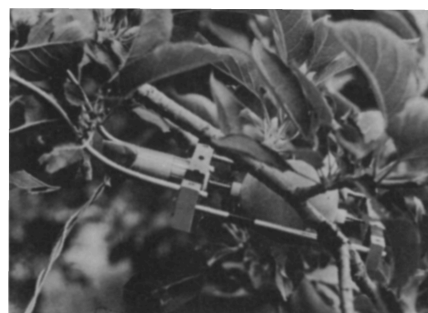
Fig. 2. Tree mounted electronic micrometer assembly.
