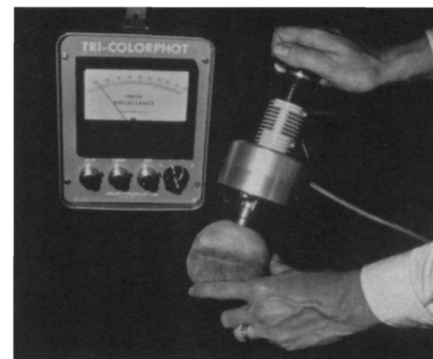
Fig. 1. New colorimeter, consisting of probe and power supply with meter.
