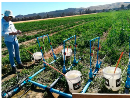
Fig. 2. Venturi injection system used for chemigation treatments in the Chilean studies.
