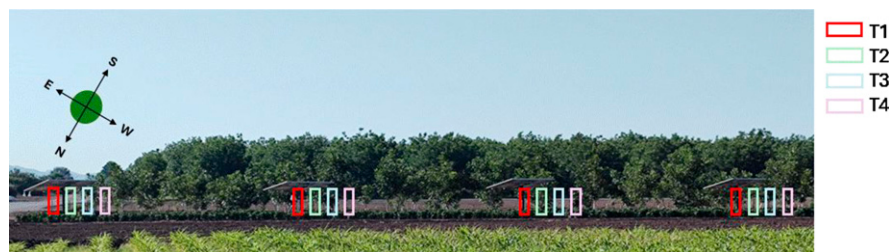
Fig. 6. The full sun replications are not shown in this image; however, their sensor setup followed the same configuration. Light sensors (Hobo Pendant MX2202; Onset, Bourne, MA, USA) were positioned at the center of each transect (T1, T2, T3, and T4) within the sample area of each photovoltaic module and full sun replication. Each sensor within the transect is represented by a color-coded rectangle for identification.
