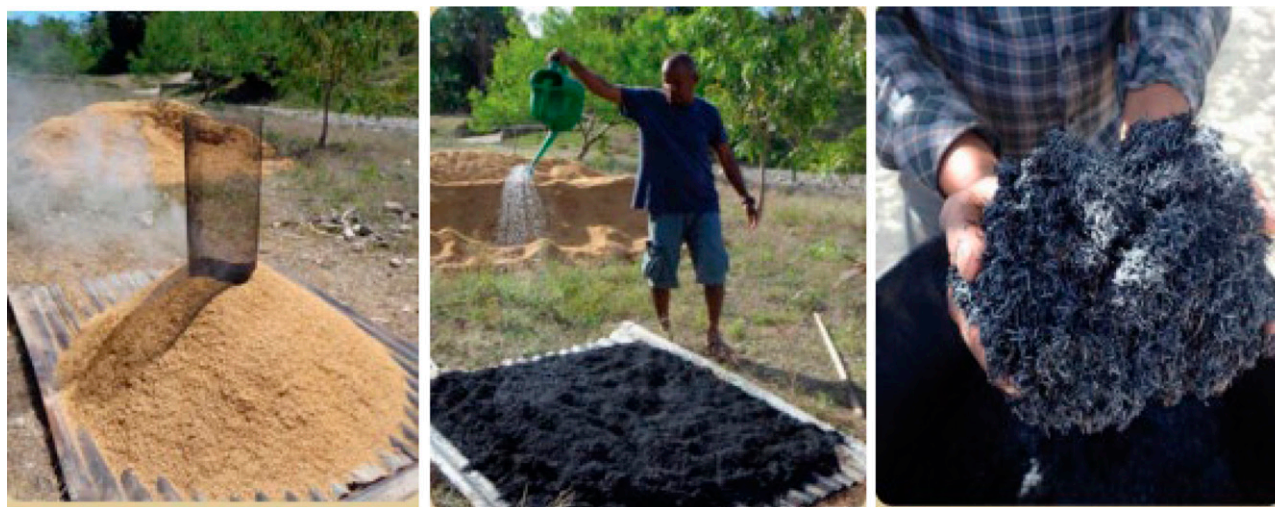
Fig. 2. Biochar production using the chimney method (source: AI-Com Timor-Leste).
