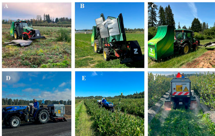
Fig. 1. Tractor-powered electrical weed control systems used in this study. (A–C) Zasso™ EH30 “Thor” (alternating current) mounted on a 77-kW tractor (5100GN; John Deere, USA). (A) Front overview in the field. (B) Close view of the front-mounted applicator head with metal electrodes (1.22-m working width). (C) Rear view showing the transformer cabinet mounted behind the tractor and driven via the power take-off. (D–F) Zasso™ XPower XPS (direct current) mounted on a 60-kW narrow orchard tractor (T4.80; New Holland, USA). (D) Front/lateral view of the unit. (E) Operation in blueberry field. (F) Rear view showing two rear-mounted applicators (0.30 m each) contacting the vegetation.
