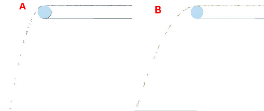
Fig. 7. The trajectory of fresh tea leaves thrown by one bud with one leaf under different transmission speeds. (A) Conveyor speed of 0.6 m/s. (B) Conveyor speed of 1.2 m/s.
