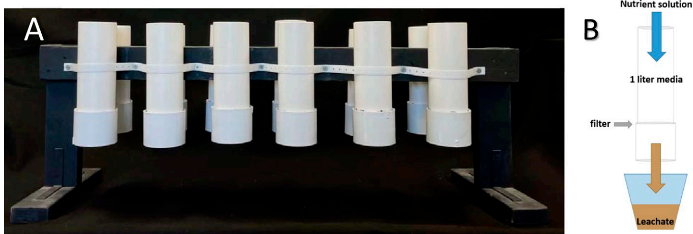
Fig. 2. A photograph of the 12 columns (1 L) used to quantify the silicon release rate in media (A) and a diagram showing leachate collection (B).
