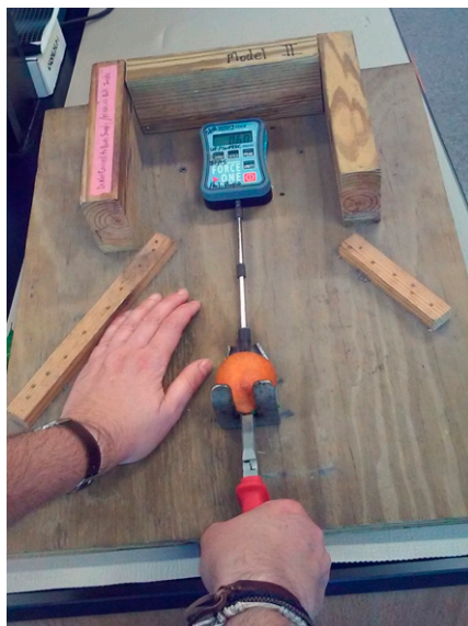
Fig. 1. Digital pull force gauge used for measuring the fruit detachment force of citrus fruits.
