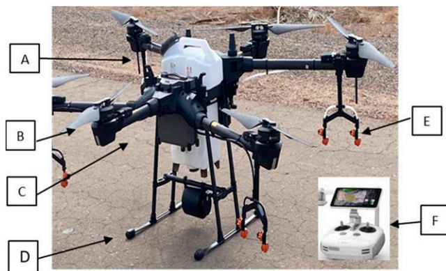
Fig. 1. The main parts of the platform-mounted robotic system (an agriculture drone DJI Agras T16) used for date palm pollination during the experimental orchard trials. Spray tank (A), propulsion system (B), battery (C), radar (D), spraying system (E), and remote controller (F).
