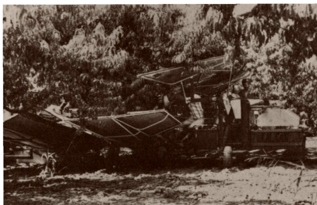
Fig. 2. Shake-catch harvester for cling peaches.
