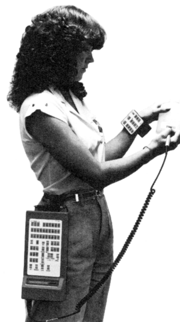
Fig. 2. Bar code symbol on a bottle scanned by an operator using a wand scanner attached to a portable decoder terminal. The decoder is hung from a belt clip to keep the operator’s hands free. Note bar-coded keyboard. A wrist band menu is worn by the operator to speed data entry of typical responses. (Photograph courtesy of Intermec Corp.).
