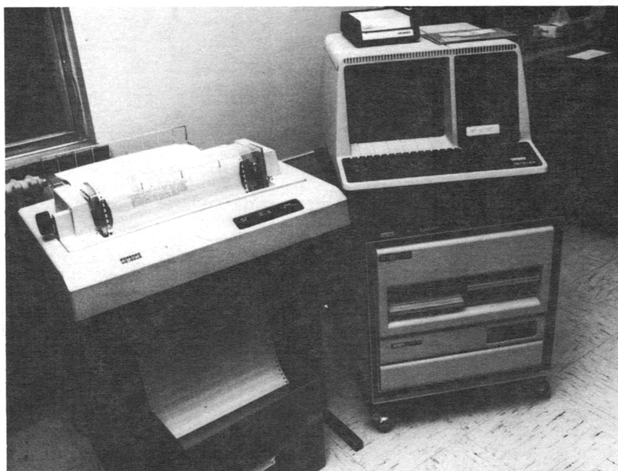
Fig. 1 The intelligent terminal included (top right) key input and video screen, (bottom right) processor, (left) printer.
