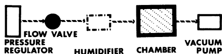
Fig. 1. Schematic diagrams of low pressure and atmospheric pressure systems. Arrows indicate direction of air flow.
