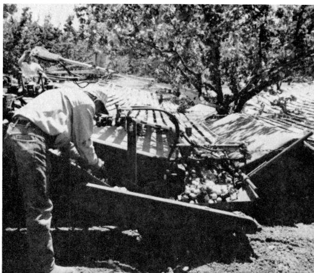
Fig. 1. Shake and catch harvester being used for apricots. Note padding and decelerator strips over the conveyor and areas of high density fruit fall. Arm of inertia limb shaker should also be padded. Limb clamp has been greatly improved over the one shown above.
