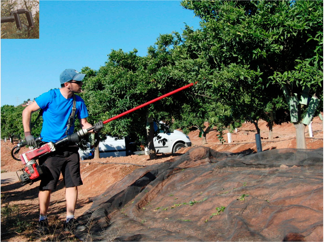
Fig. 1. Hand-held gasoline-powered shaker used for the mechanical thinning of 'Clemenrubi' mandarin and the details of the hook (upper left).
